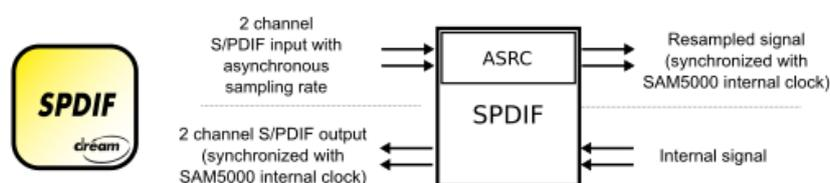
**Two channel SPDIF In/Out module with high quality Asynchronous Sample Rate Conversion (ASRC) on input to convert incoming SPDIF signal to SAM5000 internal rate.**
